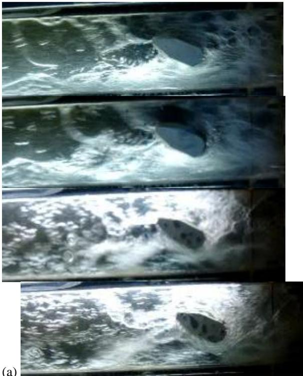
Figure 9. Photographs for the two phase flow behavior at  $Q_w=35$  l/min, angle of attack= 30 degree and  $Q_a=10, 20, 30, 40$  l/min respectively.
