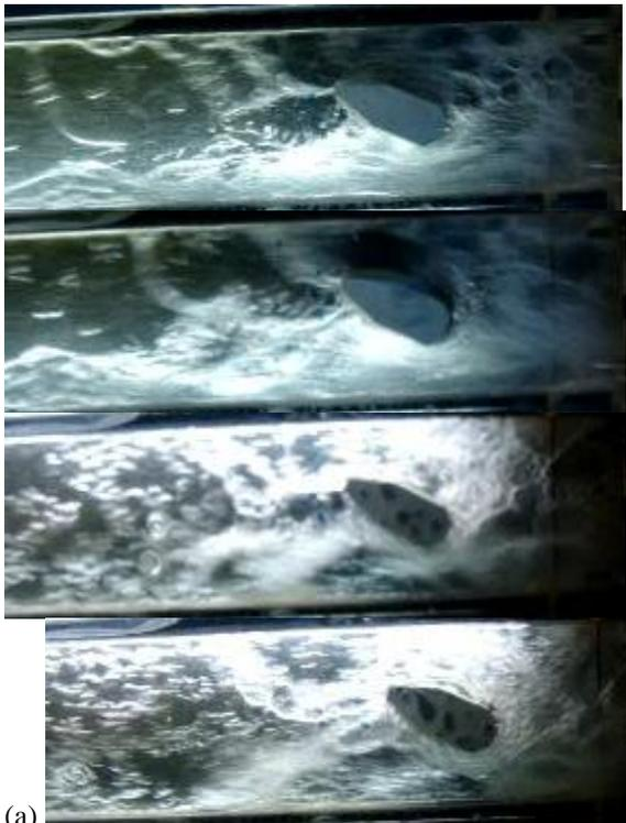
(a) Figure 9. Photographs for the two phase flow behavior at  $Q_w=35$  l/min, angle of attack= 30 degree and  $Q_a=10, 20, 30, 40$  l/min respectively.
